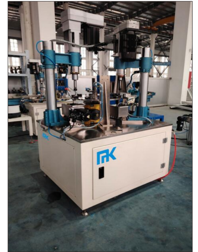
Solar Nuts Automated drilling tapping machine
